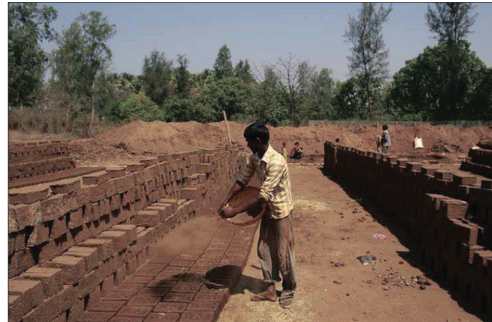
A labourer throws mud on bricks kept for drying at a kiln in Karjat, India, this month.
